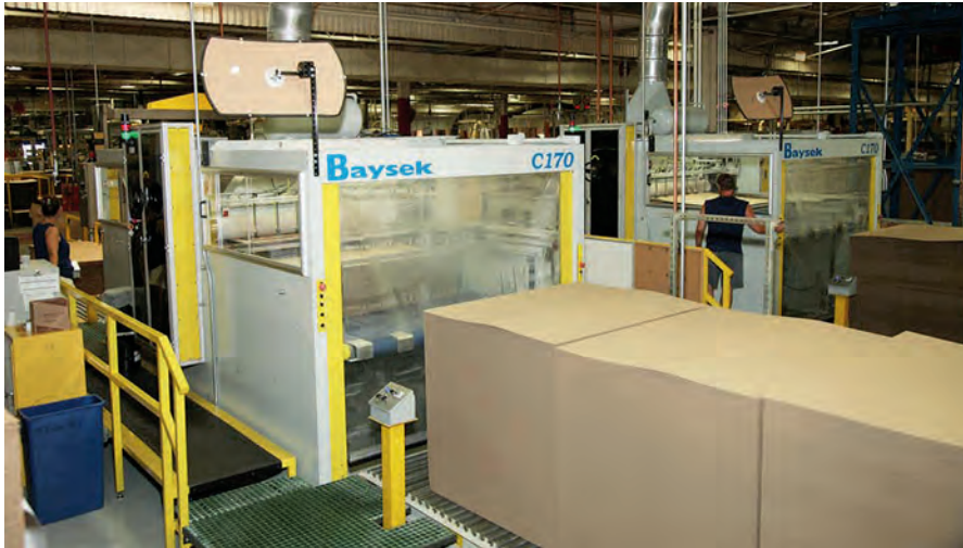
Baysek’s innovative automatic infeed (below, in blue) allows sheets to move directly from the corrugator to the two die cutters without handling.
